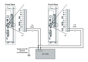
Figure 13: Multiple APS Wiring Diagram
